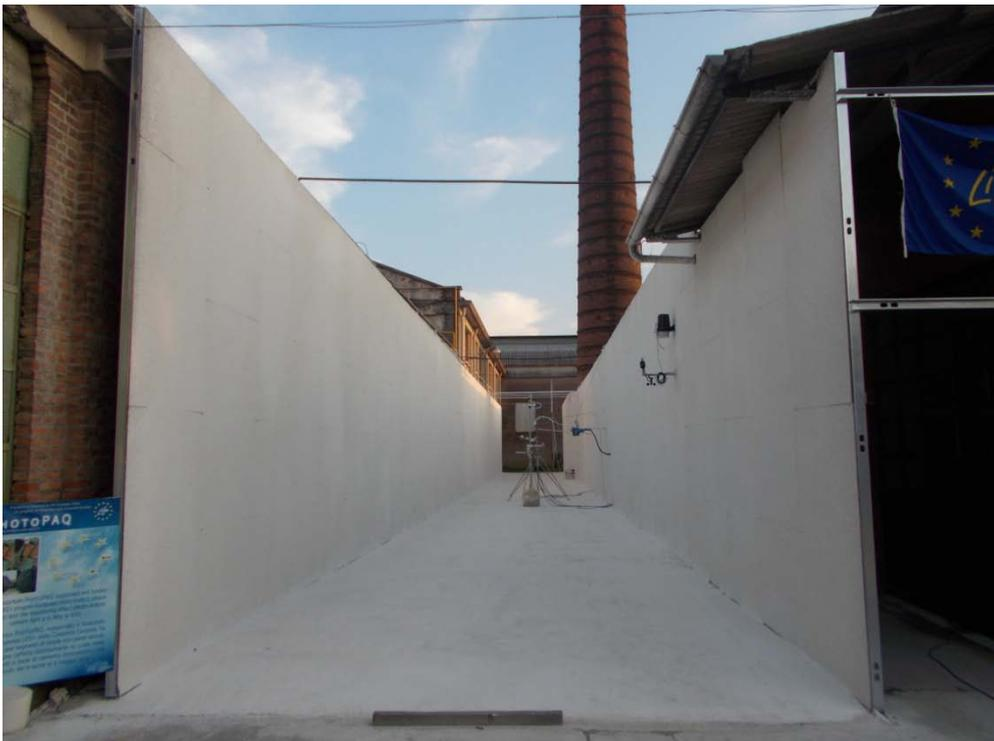
**View of the of active canyon on Petosino- Sorisole site (inlet and physical sensor can be seen on the middle)**
