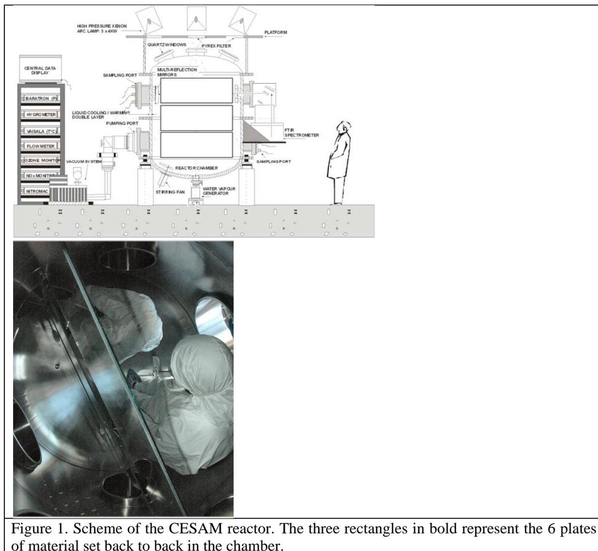
Figure 1. Scheme of the CESAM reactor. The three rectangles in bold represent the 6 plates of material set back to back in the chamber.
